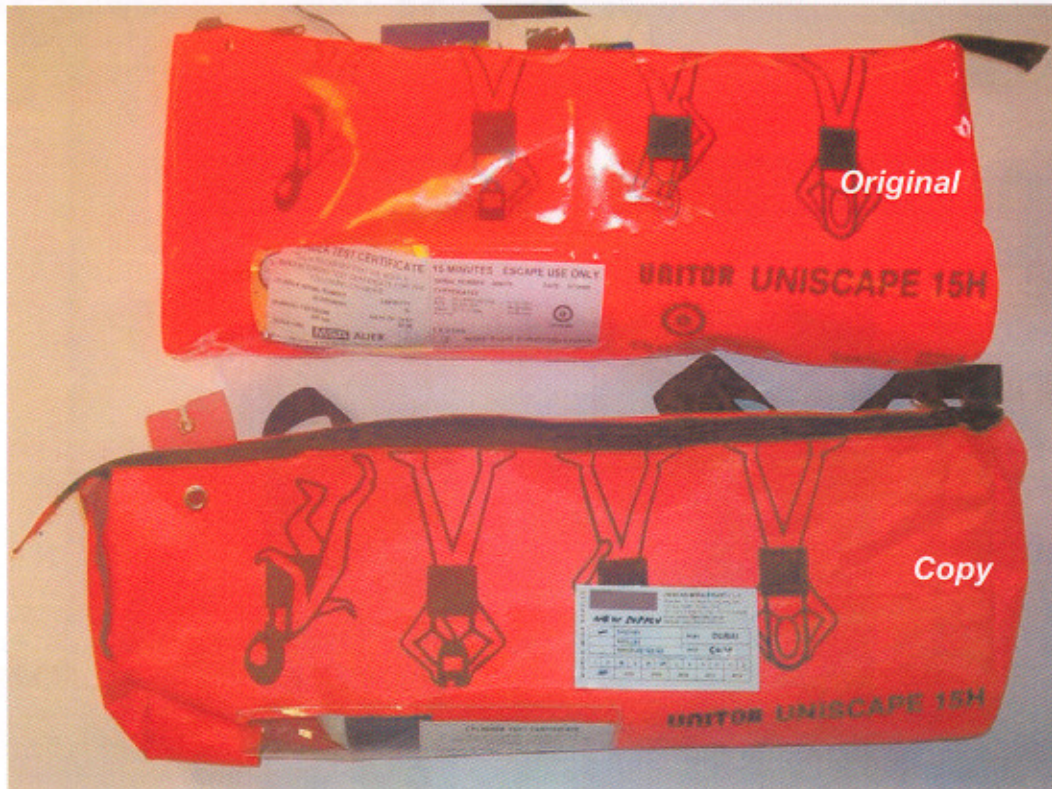
Lower: Copied equipment, with dull canvas-like material
