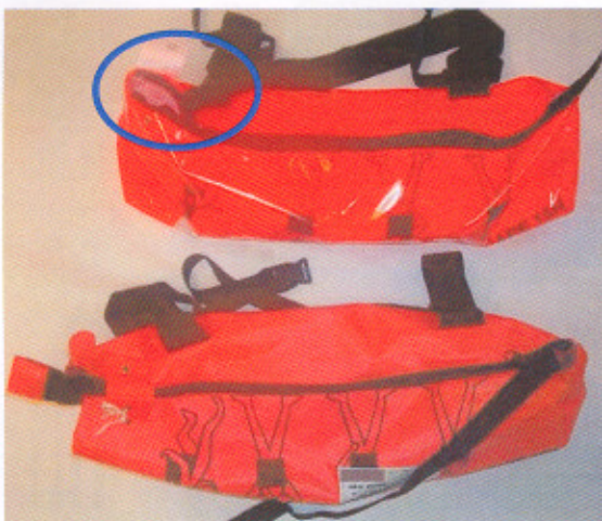
Upper: Original Unitor EEBD with shiny PVC bag
