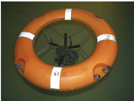
Figur 1. Livbøye testes ihht. standard flotation test
