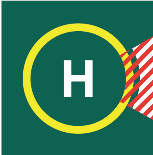
Figure 5 - Example of Prohibited Landing Heading Marking
