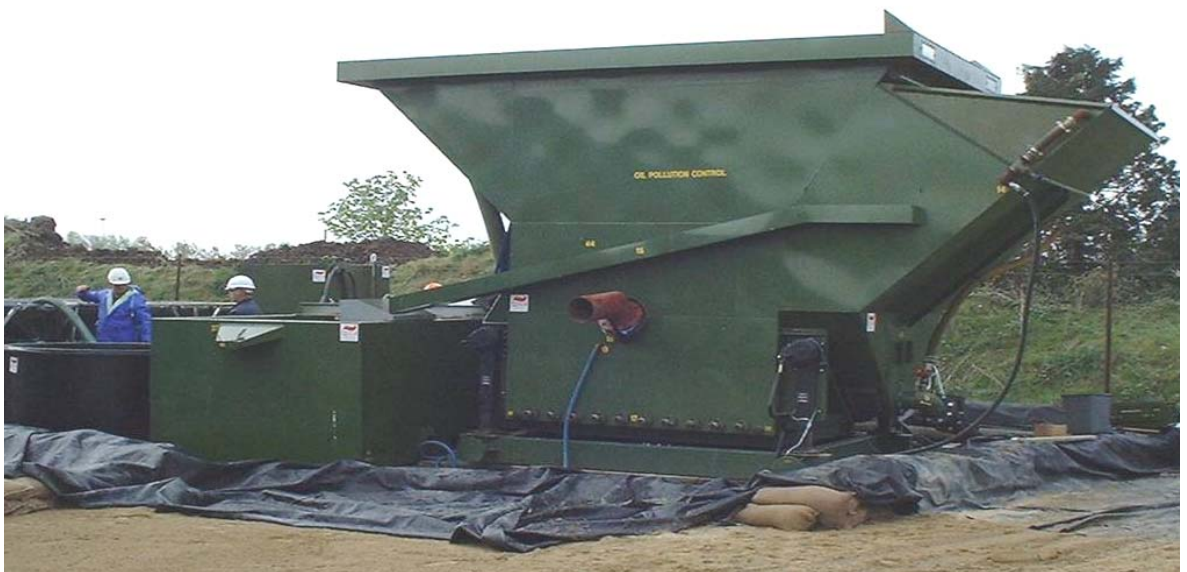
Figure 52 The Sand Scrubber
