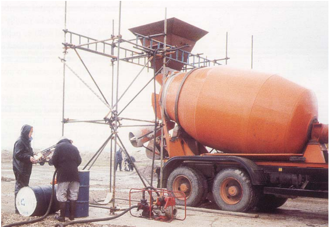
Figure 51 Hopper allowing easy loading of oiled material into the washer
