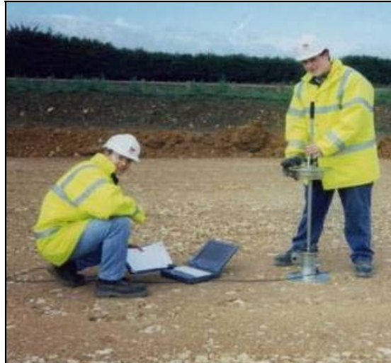
FIGURE 7.5 Lightweight Dynamic Plate Test
