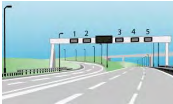
Figure 6.1: Parallel Diverge Signals
